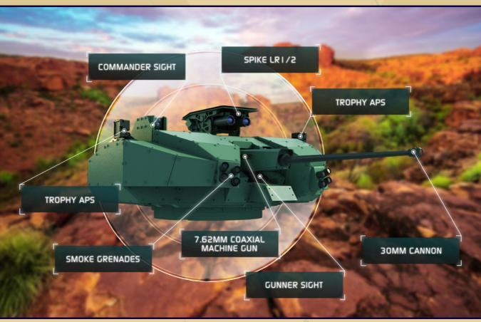
Add-On Armor STANAG LEVEL 2 | Total weight < 3.5 tons | Gun elevation: -10° to +60°
