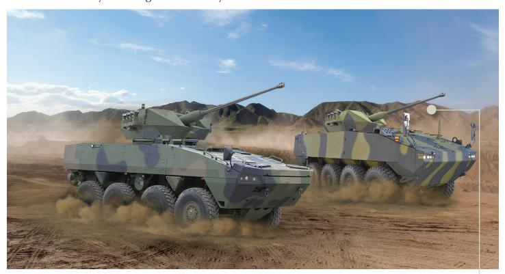
The Samson Mk II offers significant improvements, including lower silhouette, optional armor protection, and improved hit accuracy, boosted crew survivability with under-armor reloading, increased rigidity and higher gun elevation capabilities - all which enable improved combat continuity.
