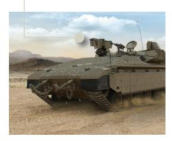
This dual-axis, gyro-stabilized RWS is designed for use on light wheeled or tracked combat vehicles, fast attack platforms requiring improved offensive capabilities. This single-weapon RWS accommodates a
