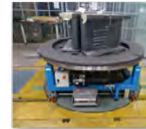
A retort propulsion system in CVD
