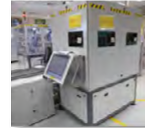
Laser welding in a closed chamber instead of TIG at the battery plant
